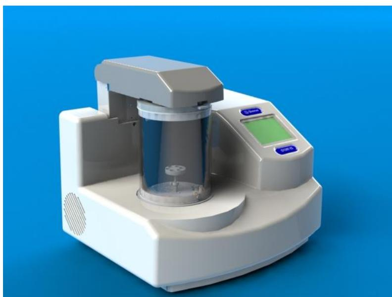
Figure 7-16. The extended height cylinder in position
